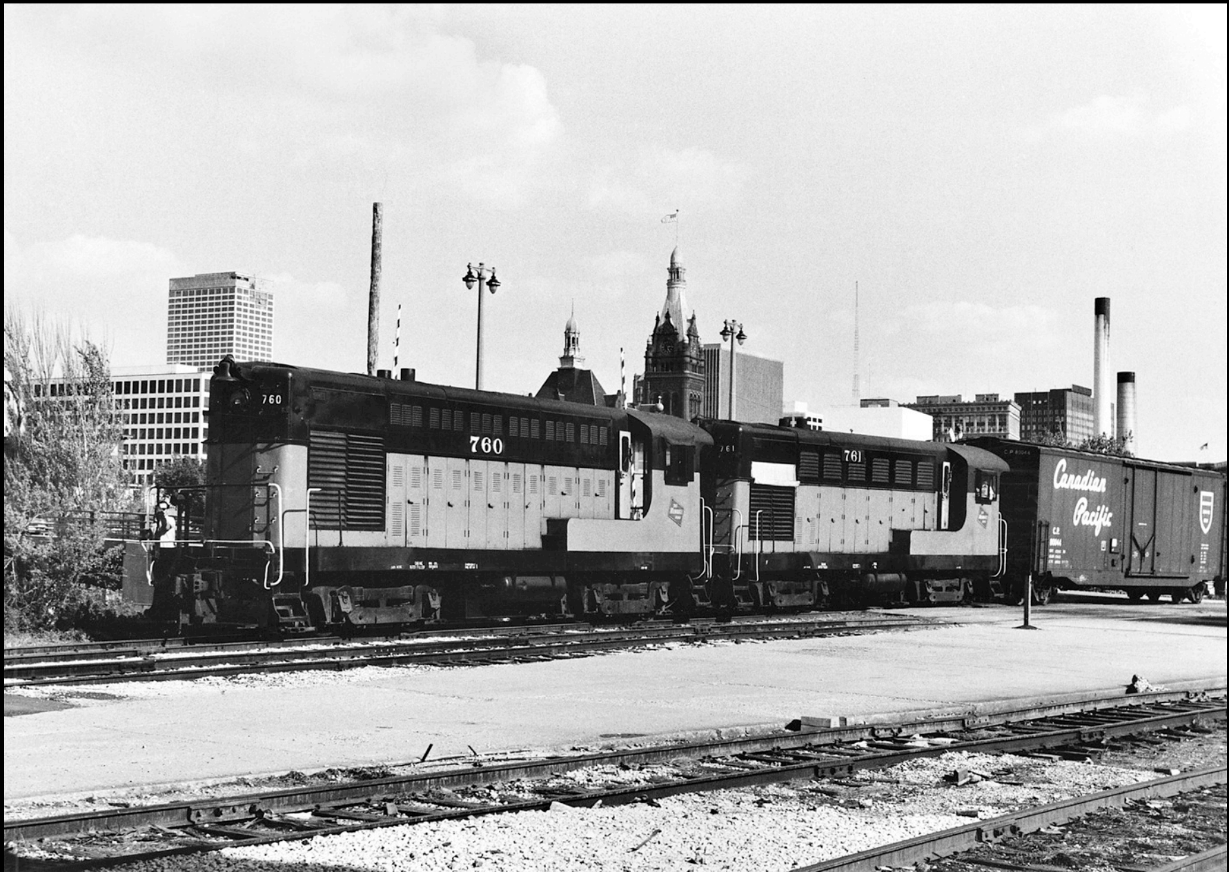
Near the end of the Beer Line at Juneau Avenue, June 1973. A pair of old Fairbanks-Morse diesels delivers newsprint to the Journal warehouse.
